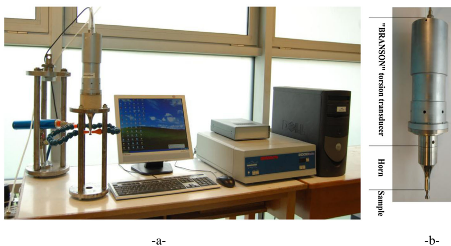
Fig. 3 a) The new ultrasonic torsion testing system; b) zoom on the transducer, the horn and the specimen.
