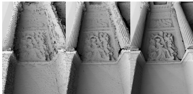
Fig. 4: Pyramidal approach: example of results during the multi-scale matching
