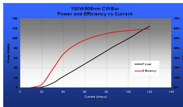
Fig. 1 – Efficiency and output power variation as function of the current absorbed from the power supply for diode lasers (Kruth, 2004).
