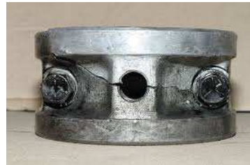
Fig.1. Failure of circular cylindrical bearing
