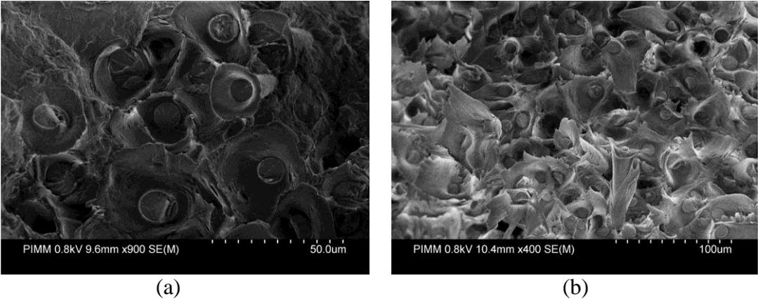
**Figure 5.** Apparition of micro-ductile areas around the fibers: (a) in the case of tension-tension fatigue test, (b) in the case of a tensile test performed at 90°C.
