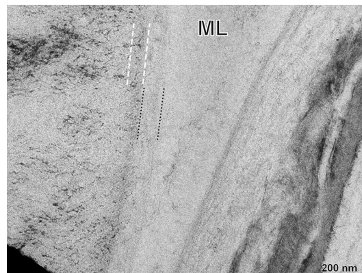
Fig. 6 High magnification TEM micrograph of the middle lamella of a flax fibre; S1 and primary cell wall are marked through two sets of dashed lines
