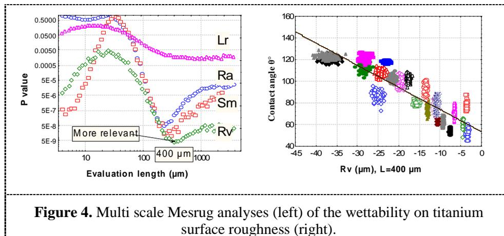
**Figure 4.** Multi scale Mesrug analyses (left) of the wettability on titanium surface roughness (right).
