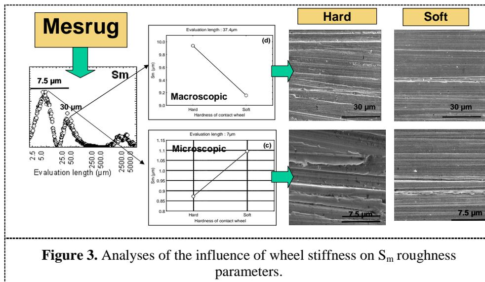
**Figure 3.** Analyses of the influence of wheel stiffness on  $S_m$  roughness parameters.
