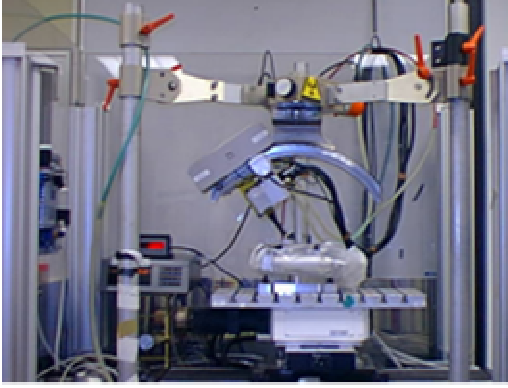
Figure 6: In-situ tensile/compressive machine placed below a SET-X diffraction goniometer
