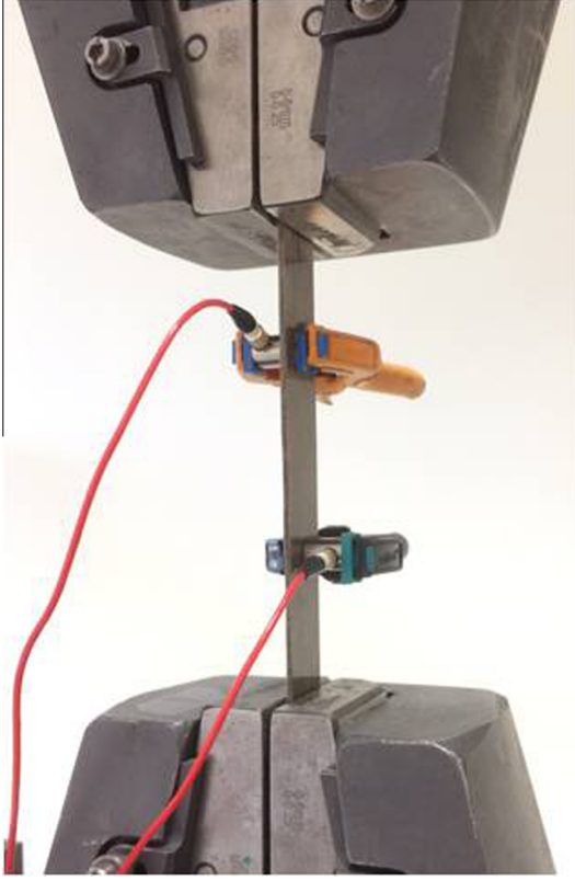
Fig. 1. Composite specimen with acoustic emission sensors. (For interpretation of the references to color in this figure legend, the reader is referred to the web version of this article.)
