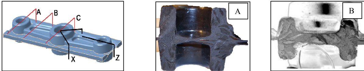
Figure 2 : Fibers displacements on two different areas A and B
