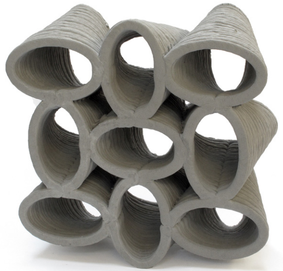
Fig. 8. Concrete 3D printed acoustic damping wall element.
