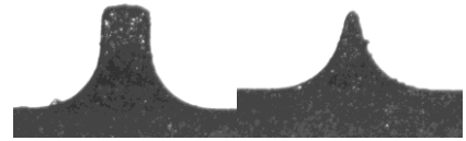
Fig. 5. Tungsten carbide tools after erosion
