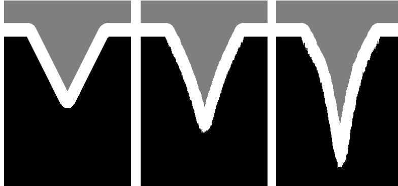
Figure 8 : Virtual cavities V_{wp} and their respective conjugate tool V_T over different iterations.
