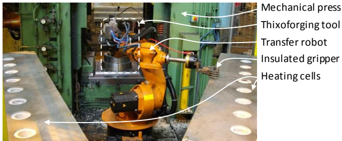
Figure 9. Semi-solid steel forging demonstrator setup in industrial plant.
