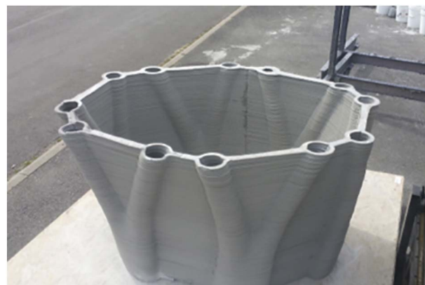
Fig. 3. Mould for a space truss (XtreeE, 2016).
