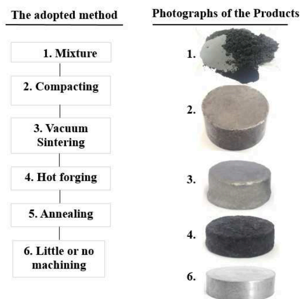
Fig. 2 Flow-chart of the adopted method and the real photographs of the product in different steps
