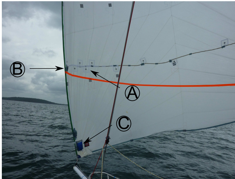
Figure 2. Photograph of the spinnaker tack. (A): tack shackle wired to the acquisition box. (B): wire running along the foot from the clew shackle to acquisition box. (C): Acquisition box with strain gauge amplifiers, a microcontroller, a wireless transmitter and a battery.
