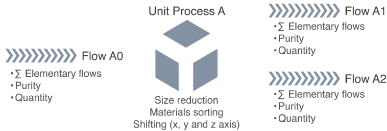
Fig. 3 Modeling of a recycling pathway step with a separation unit process
