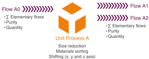
Fig. 2 Modelling of a recycling pathway step with a unit process and its related flows
