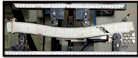
(b) Sandwich with PET foam 70 Kg/m 3 – Gridded (- res) h = 33 mm
