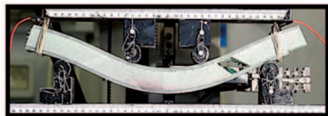
(e) Sandwich with PET foam 150 Kg/m 3 - Standard h = 33 mm
