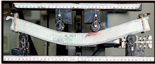
(c) Sandwich with PET foam 70 Kg/m 3 - Standard h = 33 mm
