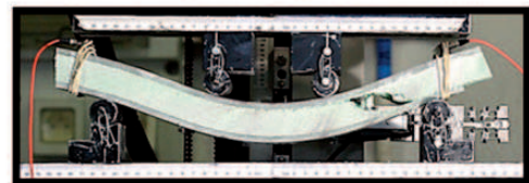
(f) Sandwich with PET foam 200 Kg/m 3 - Standard h = 33 mm
