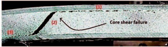
Figure 25. Typical final break on sandwiches with PET foams.
