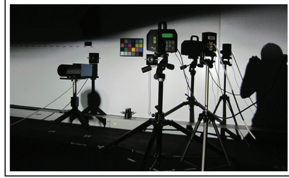
Figure 3. Real measurement conditions for the Macbeth ColorChecker chart white patch.
