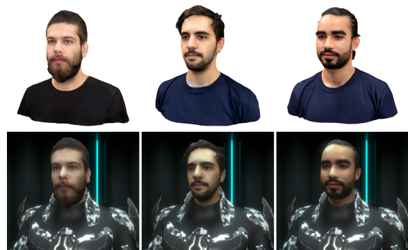
Figure 1: Illustration of three raw bust models (50K polygons) and their optimized versions (2.5K polygons) integrated in the virtual reality application
