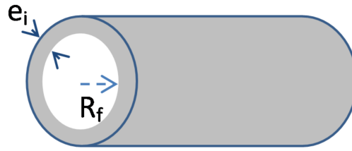
Figure 4. Schematization of a tubular interphase (in grey) around a fiber (in white area). Indication of its wall thickness and the fiber radius.
