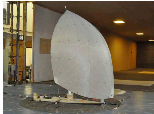
Fig. 1. Spinnaker model on the testing rig in the wind tunnel.
