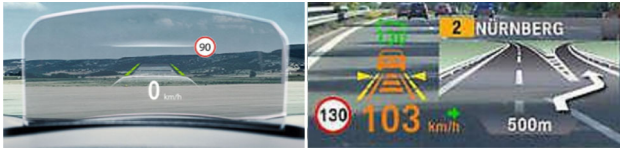
Fig. 1 HUD projections proposed by enterprise 1 and 2 [18, 28]
