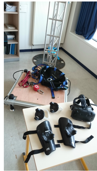
Figure 2: The WoaH simulator setup. In the foreground, the HTC Vive with the trackers to be attached to the user; in the background, the dynamic platform with the harness to be attached to the user and the real ladder fixed on a lightweight structure.
