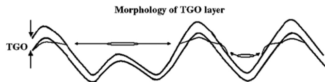
Fig. 13. Crack propagation behavior in the TBCs and its dependence on the morphology of the TGO layer and TC/BC interface [28].
