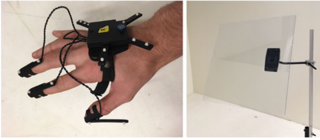
Fig. 6. A.R.T. Finger tracking device and the passive glass.
