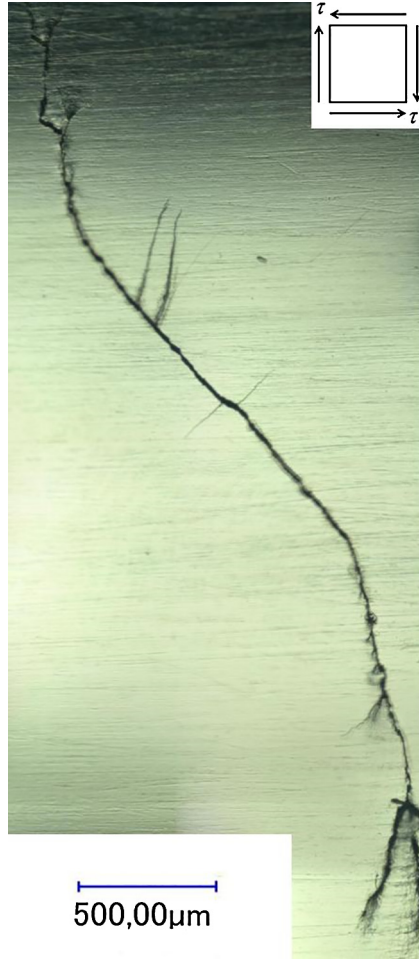
Fig. 12. Surface crack patterns in the failed specimen: \tau_a = 340 MPa; \tau_m = 500 MPa; N_{cycles} = 944,988 .
