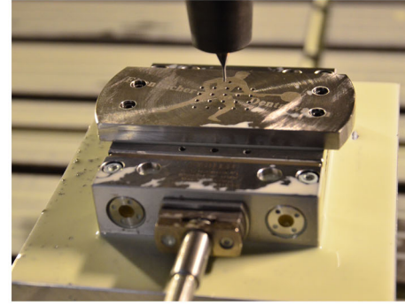
(b) Tool, Workpiece and Dynamometer
