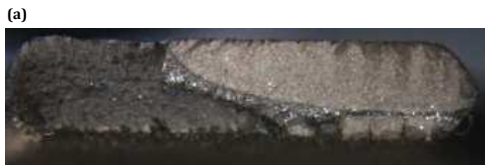
Figure 4: Fatigue fracture surface of the specimen loaded at 600 MPa (R=-1). (a) Global fracture surface showing the fatigue surface, (b) initiation zone identified at the surface of the specimen.
