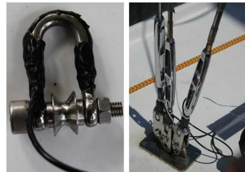
Figure 3. Gauge-fitted shackle and turnbuckles designed for the probe-fitted J80. Load cells are under the black water tight mastic.
