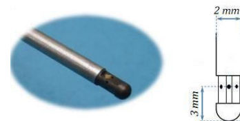
Figure 5. Sketch of the three-holes pressure probe
