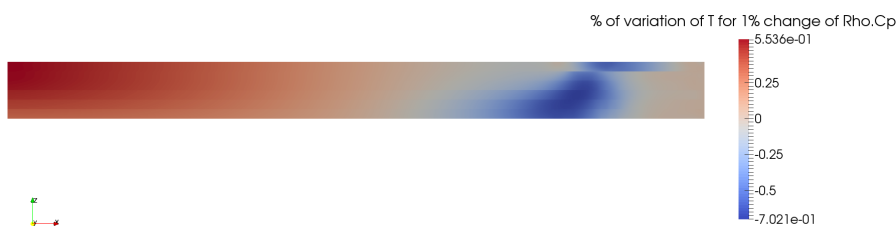
Figure 15. Temperature sensitivity with respect to \rho C_p . Variation of Temperature (in %) for a variation of 1% of the \rho C_p value. We consider the frame attached to the laying head, and consequently the right boundary corresponds to the material inlet and the left one to the outlet.
