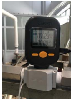
(a). Gas mass flowmeter.
