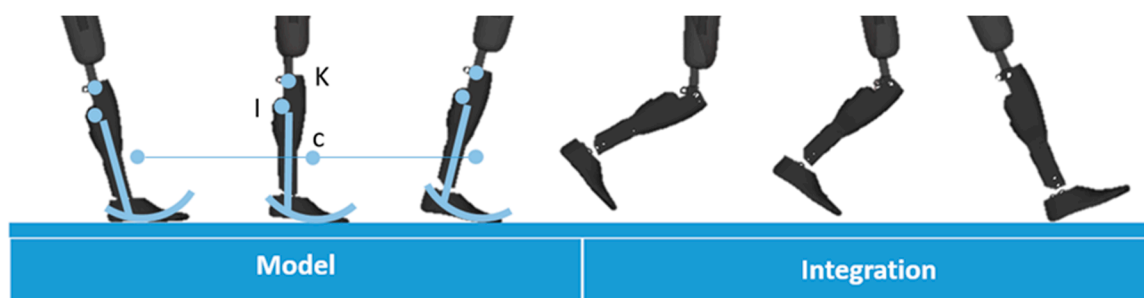
Figure 2. Computation strategy and illustration of the model used. C is the center of the curved arc foot model, K is the center of the knee, I is the center of the IMU frame.
