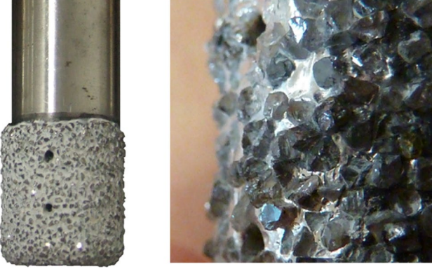
Fig. 1 Diamond abrasive cutter with grits size of 852 \mu\text{m}
