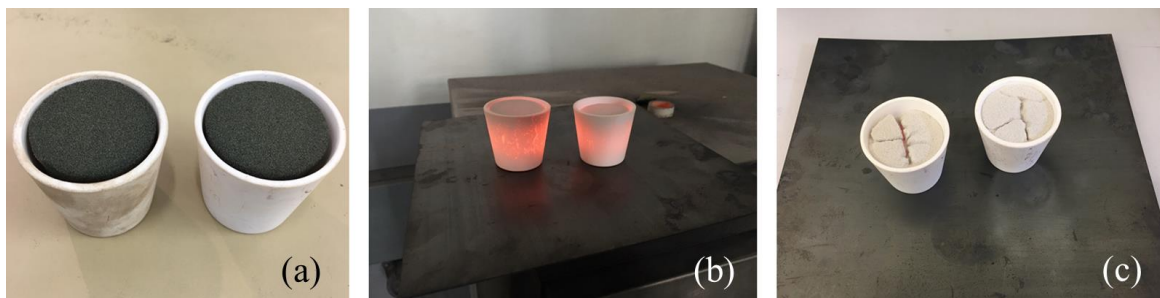
Fig.4 LOI test crucible with (a) powdered 3DP specimens,(b) immediately after taking out of the oven at 900 °C and (c) after cooling it to 150 °C, before weighting the final mass
