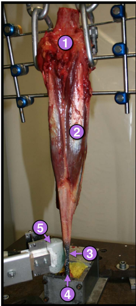
Fig. 4. Experimental set-up: anatomical specimen mounted in the material testing machine. 1. Knee, 2. Triceps surae, 3. Achilles tendon, 4. Calcaneus cemented in a bucket fixed on the testing machine, 5. Elastographic probe held by an articulated arm.
