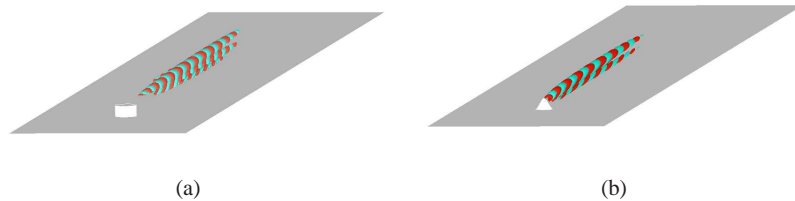
Fig. 3 Streamwise velocity component of the eigenvector of the most unstable mode obtained at Re = 1000 for the cylindrical roughness element (a) and the smooth one (b).
