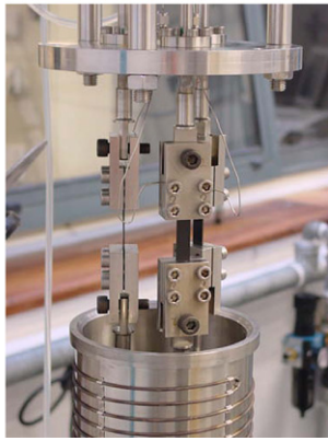
Fig. 2. Schematics and photographic image of the ENSMA COMEDI climatic chamber setup specifically developed for the thermo-oxidation testing of resin and composite samples.
