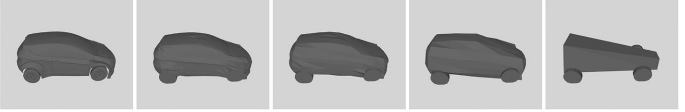
FIGURE 2 Model de-refinement for the Ford Fiesta example
