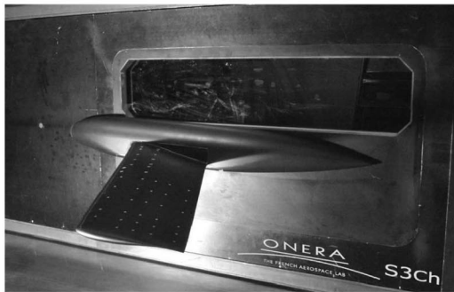
a) BUFET’N Co model in S3Ch wind tunnel
