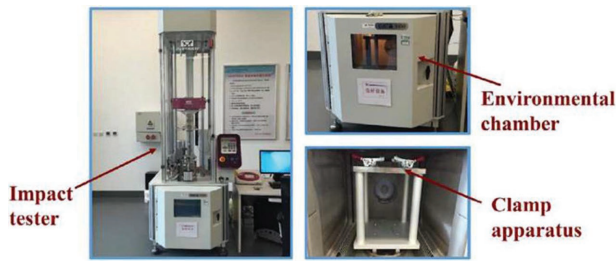
Figure 21. Experimental equipment used for low-velocity impact tests. Adapted with permission. [227] Copyright 2018, Elsevier Science Ltd.
