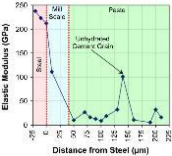
Figure 11: Evolution of elastic modulus across the ITZ between concrete and bare steel [27].
