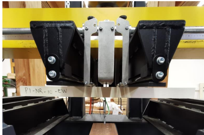
Figure 8. LVL poplar beam during bending test.
