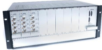
Figure 2: Up to 36 PZT channels simultaneously emitting or receiving signals with 1 \mu s selective commutation
