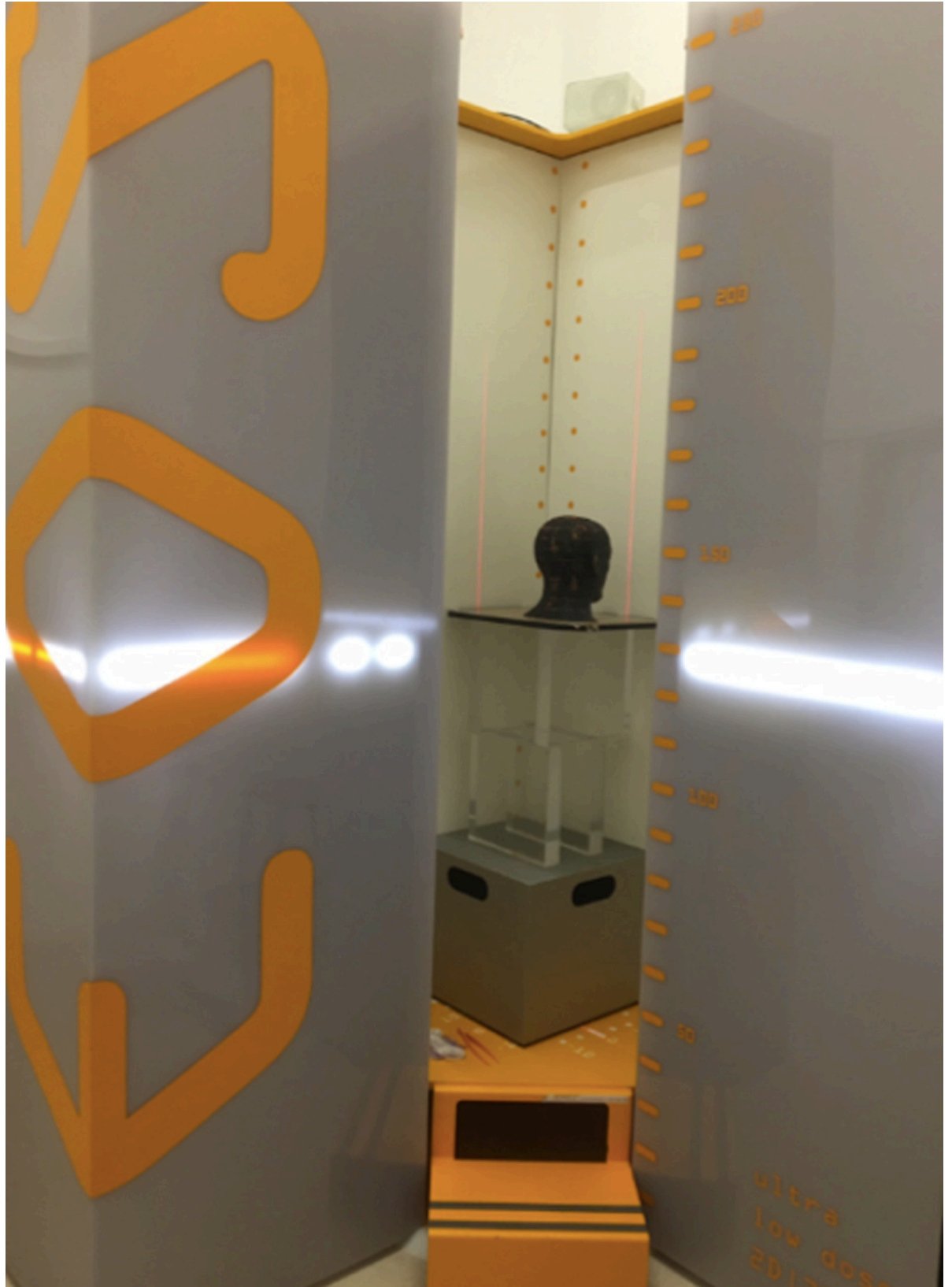
Fig 3. For better illustration, an Alderson head phantom was placed in the biplanar low-dose X-ray imaging system. The light outside is a laser beam, showing the height in which the image is captured at this moment. A certain distance (in cm) can be set in the system.
