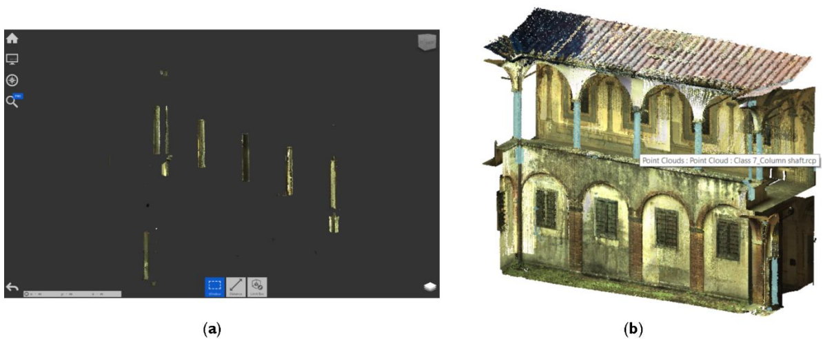
Figure 14. Label 7—Column shaft imported into Recap upfront (a) and later selected on the overall point cloud in Revit (b).
