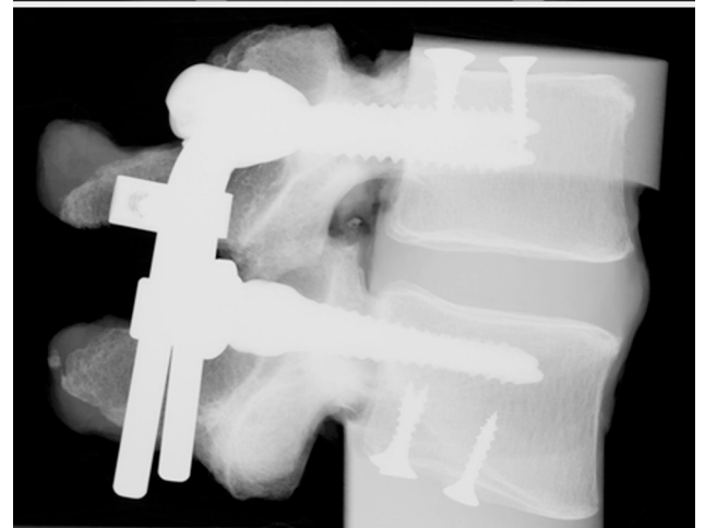
Fig. 5. Antero-posterior and lateral radiographs of instrumented L4-L5 segment with lesion and vertebral bodies embedded in Poly Methyl MethAcrylate (PMMA).
